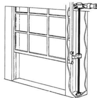
Automatic switch on large windows (doors)
